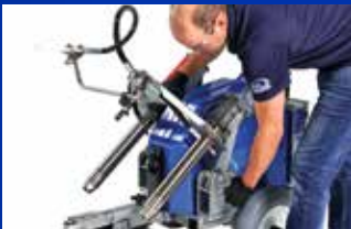
2) Tilt pump assembly back
