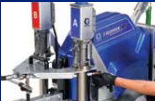
1) Remove retaining clamps and pressure transducer connections
