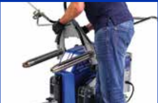
3) Remove ProConnect Pumping System
